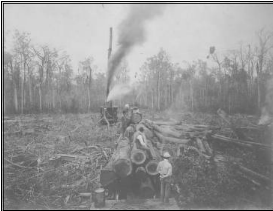
Figure 81. Logging operation showing logs on tram cars and small portable steam engine.
