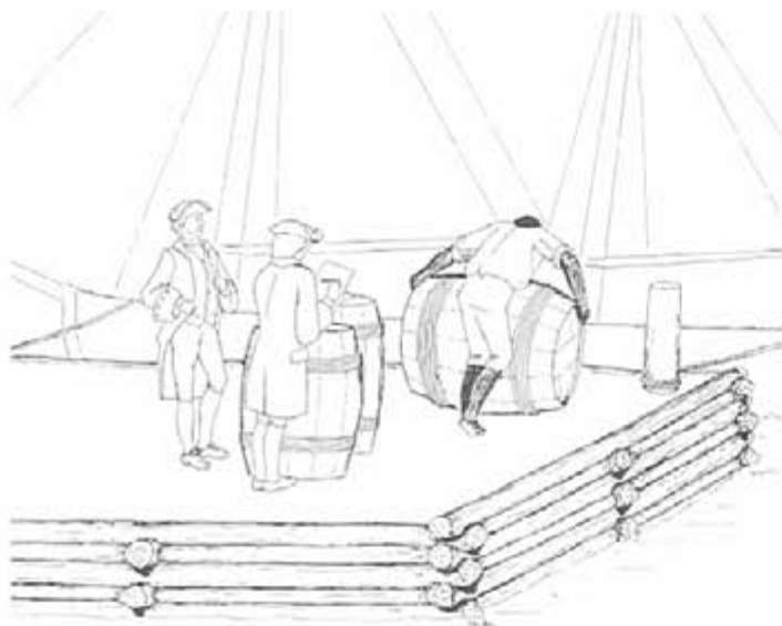
Dorchester's cribwork log wharves, one of which is shown here in a conjectural reconstruction, apparently were a response to local geology: A rock-hard marl river bottom made driving piles a difficult, if not impossible, task.
