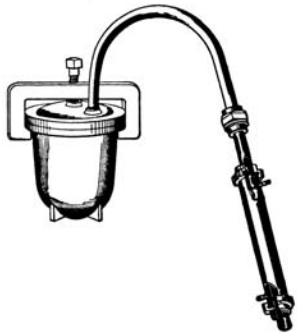
Figure 25. Pot Retort. The Casing at the Lower End of the Tube is the Water Jacket For Condensing the Mercury Vapor (Richards 1909).
