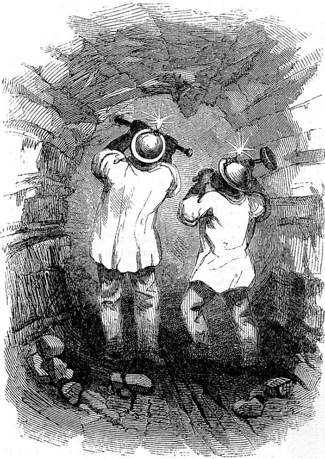
Figure 5. African-American Miners Drilling Holes for Blasting in a North Carolina Gold Mine (Harpers 1857).
