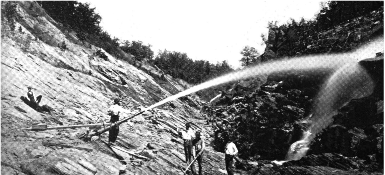
Figure 39. Hydraulic Placer Mining Produced Distinctive Features Such As a Washed Out Bank and Sluice. Unknown Location, Carolinas or Gerogja (Source: Nitze & Wilkens 1896).
