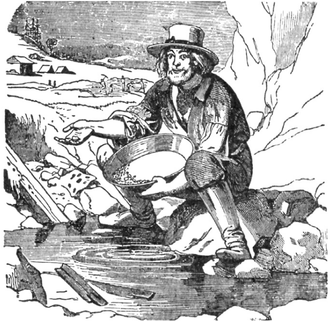
Figure 7. Panning was an Important Prospecting Method (Rickard 1932).
